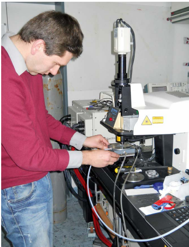
Abb. 49: Dr. Robert Lehmann at the Leibniz Universität Hannover preparing for lead isotope analysis of coins with fs-LA-ICP-MS; Photo: S. Merkel.
