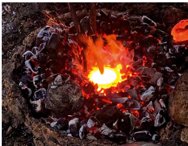
Abb. 48-49: Partly-fused melted masses of copper prills in-between and surrounding charcoal following the conversion of malachite > copper oxide > copper metal within simple reducing pit furnaces.
