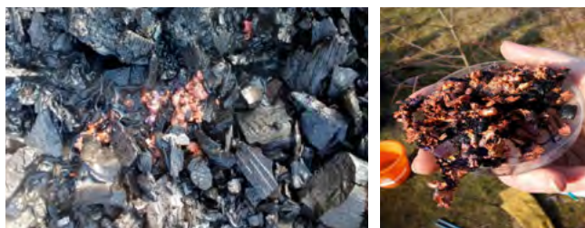
Abb. 48-49: Partly-fused melted masses of copper prills in-between and surrounding charcoal following the conversion of malachite > copper oxide > copper metal within simple reducing pit furnaces.
