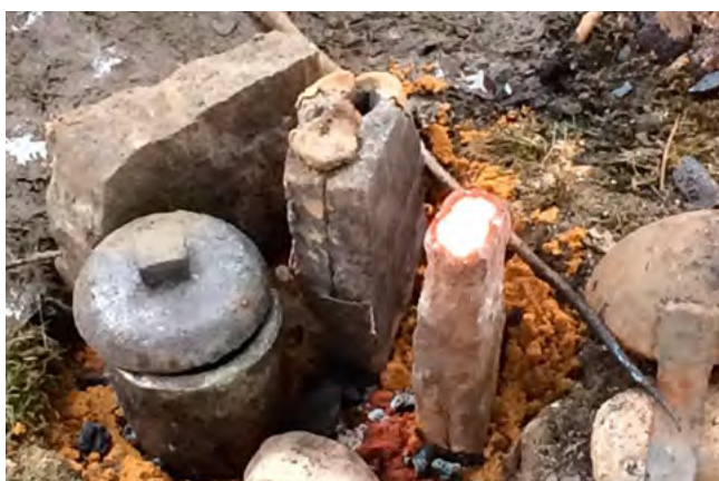
Abb. 52: Detail of cooling bronze melt within the top of the sprue cup of the clay mould. The bivalve stone mould for the EBA bronze dagger stands next to this.
