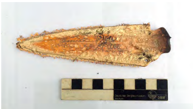
Abb. 53-54: Rough EBA knife casting as just removed from bivalve mould (with flashing intact). Removing the flashing and surface roughness of the metal using water and sand on a grindstone.
