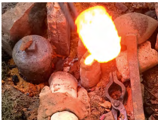
Abb. 50-51: Bowl furnace used for copper/bronze melting – opened up and top of crucible revealed at 1200°C. The pouring of bronze into closed clay mould.
