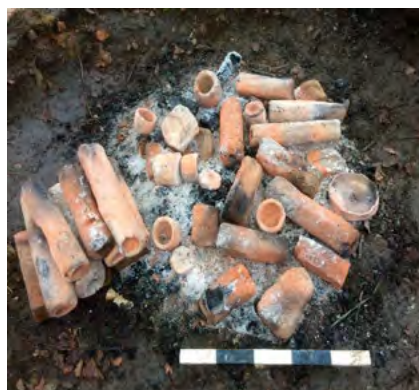
Abb. 45-46: Firing hand-made clay tuyere pipes, crucibles, pots, stands and clay moulds within an open bonfire-type kiln (Bronze Age-type firing) in a wood fire at temperatures of between 800-950°C.
